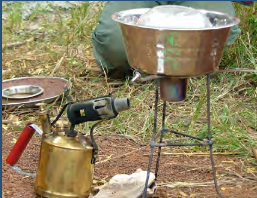
A locally fabricated retort
