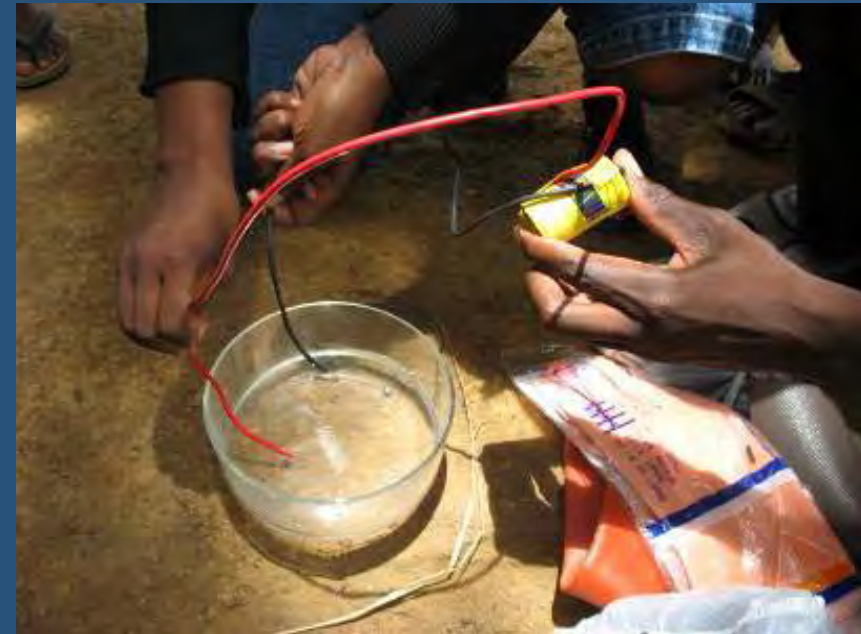
Miner re-activating mercury using a radio battery; the process takes about 10 - 20 minutes
