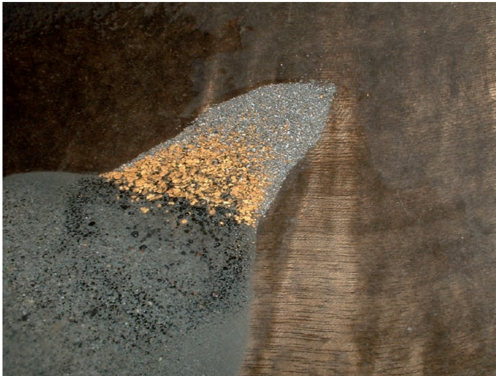
Gold and platinum at the bottom of a pan © R De Hommel
